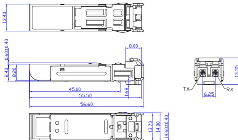
**DIMENSIONS ARE IN MILLIMETERS**
