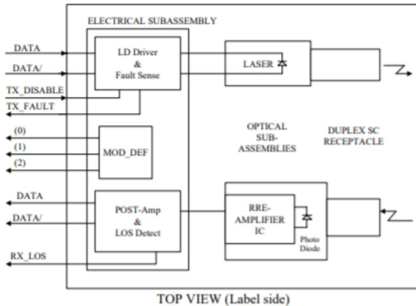
**Transmitter Section** - The transmitter section consists of a 1310 nm InGaAsP laser in an eye safe optical subassembly (OSA) which mates to the fiber cable. The laser OSA is driven by a LD driver IC which converts differential input LVPECL logic signals into an analog laser driving current.
