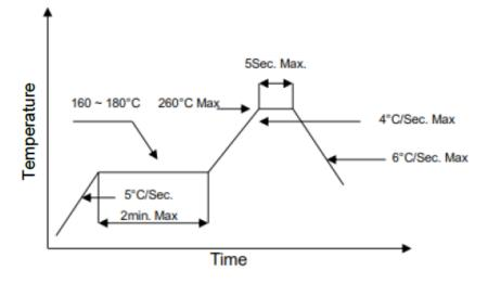
Note: Reflow soldering can be operated only one time. During the temperature ramp-up, no forces may be exerted on the LD which would deform or damage them. After soldering is completed, please do not process until the product temperature ramps down to room temperature.
