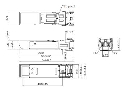
DIMENSIONS ARE IN MILLIMETERS
