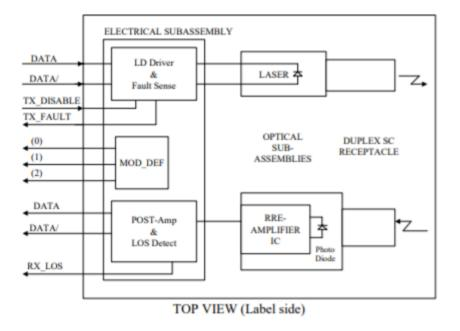
**Transmitter Section** - The transmitter section consists of a 1550 nm InGaAsP laser in an eye safe optical subassembly (OSA) which mates to the fiber cable. The laser OSA is driven by a LD driver IC which converts differential input LVPECL logic signals into an analog laser driving current.
