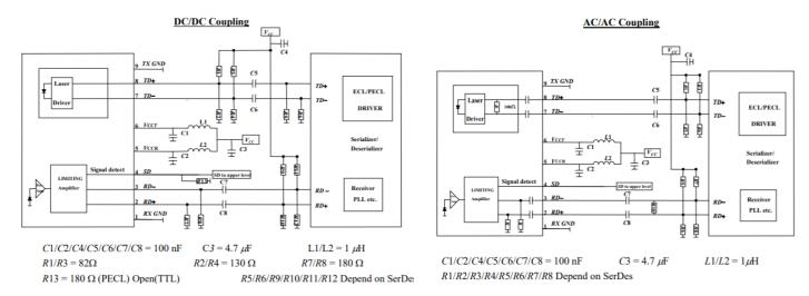
In order to get proper functionality, a recommended circuit is provided in above recommended circuit schematic. When designing the circuit interface, there are a few fundamental guidelines to follow.
