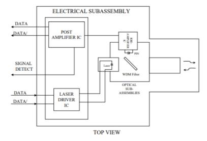
Transmitter and Receiver Optical Sub-Assembly Section - A 1310 nm InGaAsP laser and an InGaAs PIN photodiode integrate with an WDM filter to form a bi-directional single fiber optical subassembly (OSA). The laser of OSA is driven by a LD driver IC which converts differential input LVPECL logic signals into an analog laser driving current. The photodiode of OSA is connected to a circuit providing post-amplification quantization, and optical signal detection.
