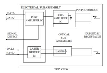
**Transmitter Section** - The transmitter section consists of a 1550 nm InGaAsP in an eye safe optical subassembly (OSA) which mates to the fiber cable. The laser OSA is driven by a LD driver IC which converts differential input PECL logic signals into an analog laser driving current.
