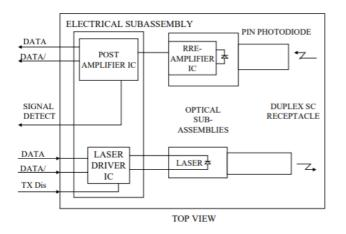
**Transmitter Section** - The transmitter section consists of a 1550 nm laser in an eye safe optical subassembly (OSA) which mates to the fiber cable. The laser OSA is driven by a LD driver IC which converts differential input LVPECL logic signals into an analog laser driving current.
