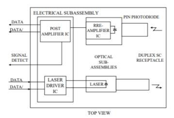
**Transmitter Section** - The transmitter section consists of a 1550 nm InGaAsP laser in an eye safe optical subassembly (OSA) which mates to the fiber cable. The laser OSA is driven by a LD driver IC which converts differential input LVPECL logic signals into an analog laser driving current.
