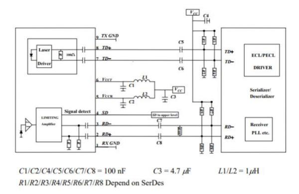
In order to get proper functionality, a recommended circuit is provided in above recommended circuit schematic. When
