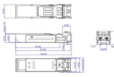
DIMENSIONS ARE IN MILLIMETERS ALL DIMENSIONS ARE ± 0.2mm UNLESS OTHERWISE SPECIFIED
