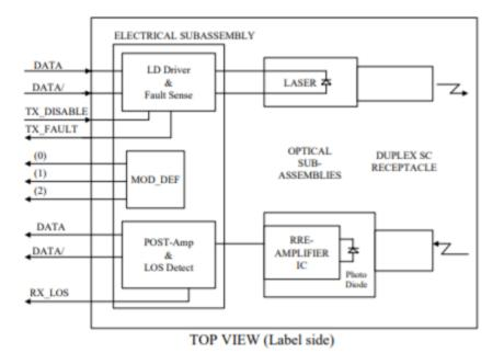
**Transmitter Section** - The transmitter section consists of a 1310 nm InGaAsP laser in an eye safe optical subassembly (OSA) which mates to the fiber cable. The laser OSA is driven by a LD driver IC which converts differential input LVPECL logic signals into an analog laser driving current.
