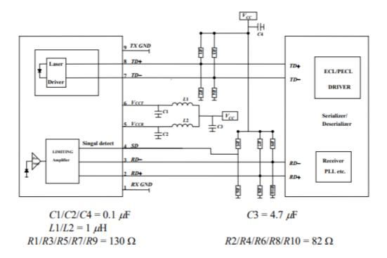
In order to get proper functionality, a recommended circuit is provided in above recommended circuit schematic. When designing the circuit interface, there are a few fundamental guidelines to follow.
