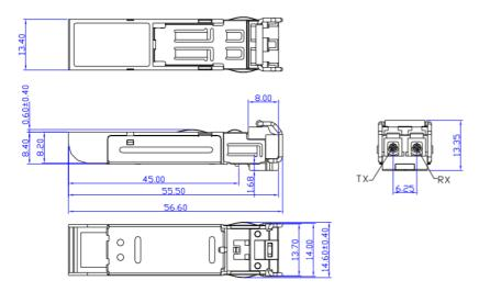
DIMENSIONS ARE IN MILLIMETERS
