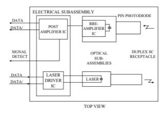
**Transmitter Section** - The transmitter section consists of a 1550nm InGaAsP in an eye safe optical subassembly (OSA) which mates to the fiber cable. The laser OSA is driven by a LD driver IC which converts differential input PECL logic signals into an analog laser driving current.
