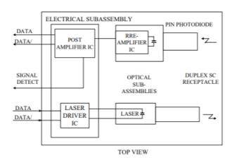
**Transmitter Section** - The transmitter section consists of a 1310nm InGaAsP in an optical subassembly (OSA) which mates to the fiber cable. The laser OSA is driven by a LD driver IC which converts differential input PECL logic signals into an analog laser driving current.
