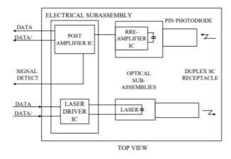
**Transmitter Section** - The transmitter section consists of a 1310nm InGaAsP in an eye safe optical subassembly (OSA) which mates to the fiber cable. The laser OSA is driven by a LD driver IC which converts differential input PECL logic signals into an analog laser driving current.
