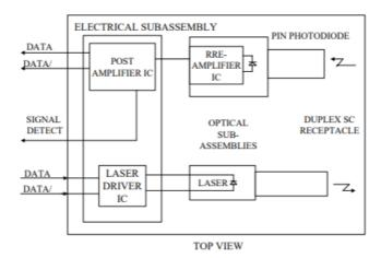
**Transmitter Section** - The transmitter section consists of a 1310nm InGaAsP in an eye safe optical subassembly (OSA) which mates to the fiber cable. The laser OSA is driven by a LD driver IC which converts differential input LVPECL logic signals into an analog laser driving current.
