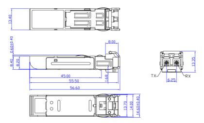
DIMENSIONS ARE IN MILLIMETERS
