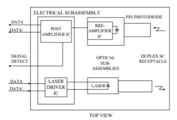
**Transmitter Section** - The transmitter section consists of a 1310nm InGaAsP in an optical subassembly (OSA) which mates to the fiber cable. The laser OSA is driven by a LD driver IC which converts differential input PECL logic signals into an analog laser driving current.
