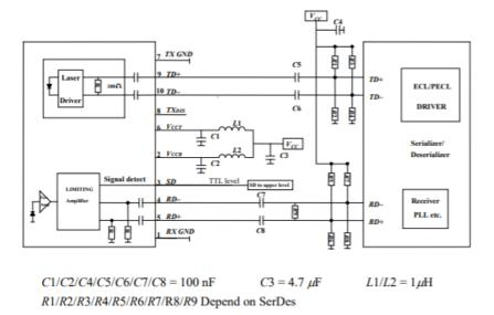
In order to get proper functionality, a recommended circuit is provided in above recommended circuit schematic. When designing the circuit interface, there are a few fundamental guidelines to follow.
