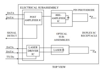
**Transmitter Section** - The transmitter section consists of a 850 nm laser in an eye safe optical subassembly (OSA) which mates to the fiber cable. The laser OSA is driven by a LD driver IC which converts differential input LVPECL logic signals into an analog laser driving current.
