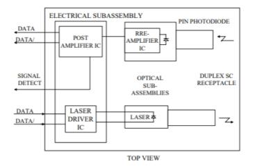
**Transmitter Section** - The transmitter section consists of a 850 nm laser in an eye safe optical subassembly (OSA) which mates to the fiber cable. The laser OSA is driven by a LD driver IC which converts differential input LVPECL/PECL logic signals into an analog laser driving current.
