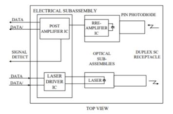
**Transmitter Section** - The transmitter section consists of a 850 nm VCSEL in an eye safe optical subassembly (OSA) which mates to the fiber cable. The laser OSA is driven by a LD driver IC which converts differential input LVPECL logic signals into an analog laser driving current.
