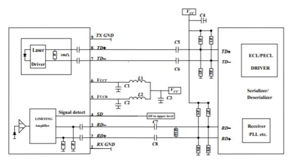
C1/C2/C4/C5/C6/C7/C8 = 100 nF  $C3 = 4.7 \ \mu\text{F}$ R1/R2/R3/R4/R5/R6/R7/R8 Depend on SerDes  $L1/L2 = 1\mu H$
