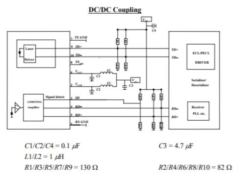
In order to get proper functionality, a recommended circuit is provided in above recommended circuit schematic. When designing the circuit interface, there are a few fundamental guidelines to follow.
